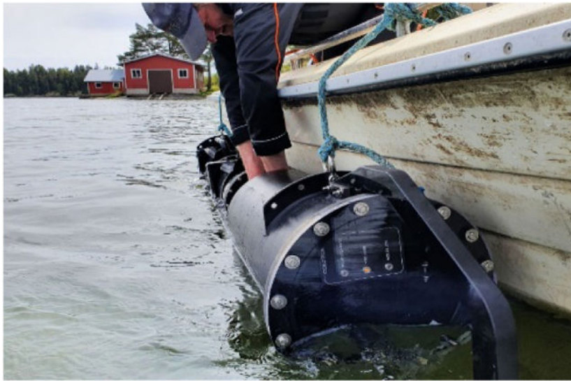
Fig. 4. On the left the mobile ADD along the side of a fishing boat. Photo: Esa Lehtonen. On the right a schematic drawing of a mobile ADD housing. The deterrent is placed at the bottom of the housing. Source: Modul Plastic Oy.
