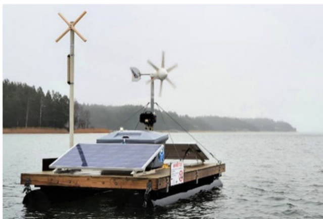
Fig. 3. Raft carrying an ADD unit and outfitted with solar panels and a wind generator for charging the batteries. Photo: Esa Lehtonen.
