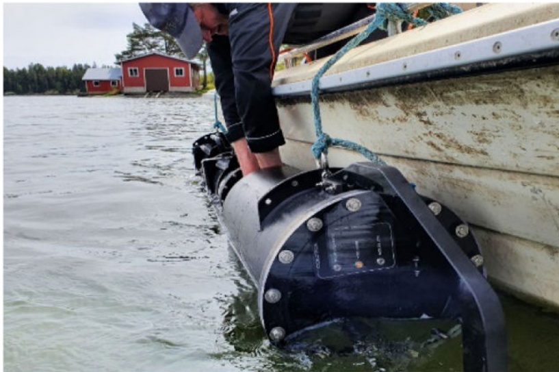
Fig. 4. On the left the mobile ADD along the side of a fishing boat. Photo: Esa Lehtonen. On the right a schematic drawing of a mobile ADD housing. The deterrent is placed at the bottom of the housing.
